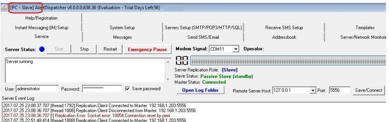
The following screen will be shown if the Passive Slave is disconnected from the Active Master. The Passive Slave status will then change to "failover" which means all messages sent to it will be processed.
