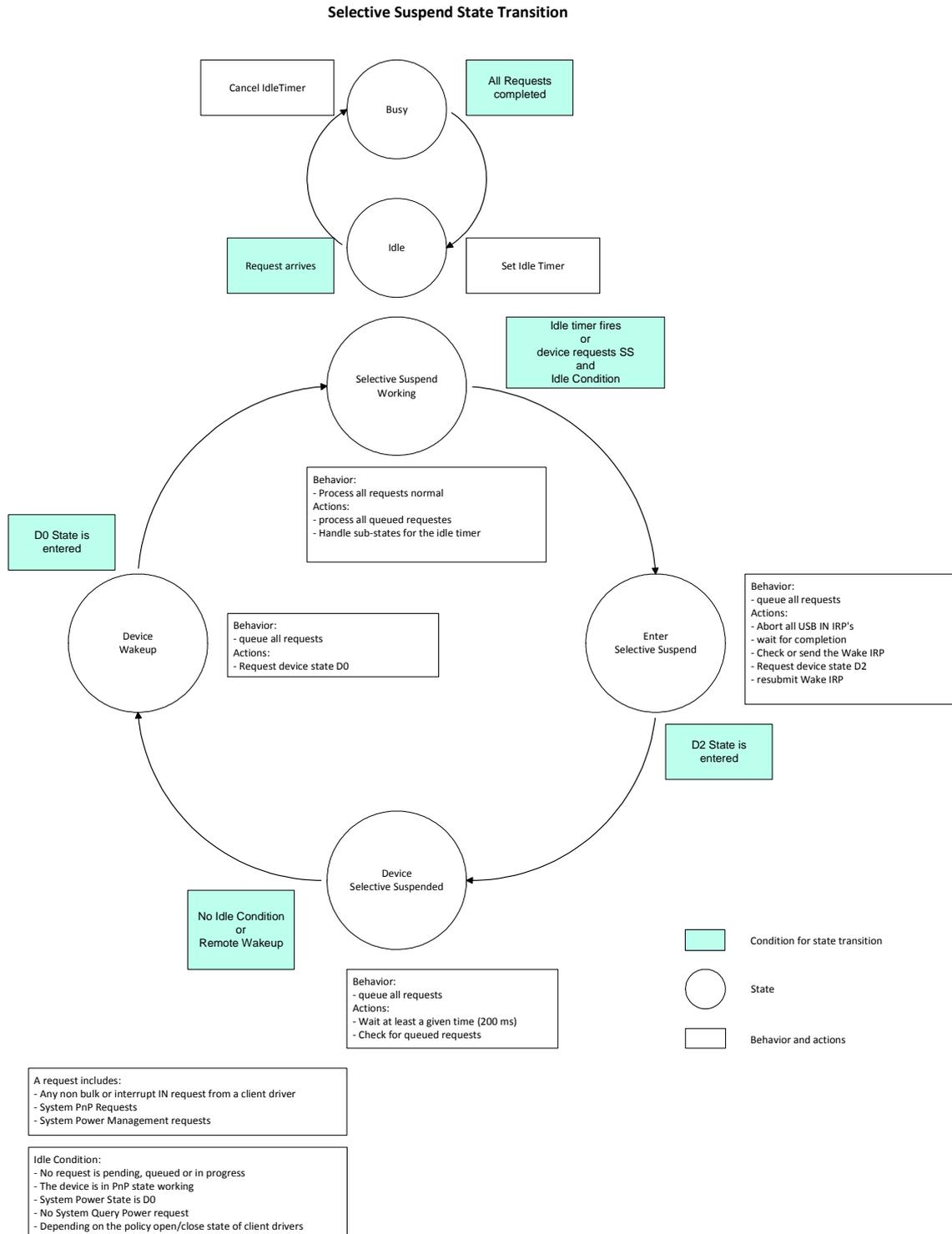
The state transition to selective suspend can be blocked if either the CDCACM is driver is opened or if the Network adapter reports a connected Network Cable.
