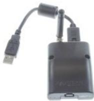
After installing the driver, insert the SIM card\* and then connect the modem to an available USB port. If Windows “Add New Hardware Wizard” appears, please direct Windows to find the driver under c:\Windows\System32\Drivers. If you are using Vista or 7 or 2007, the driver should be automatically detected. The modem should light up after the driver has been properly installed.
