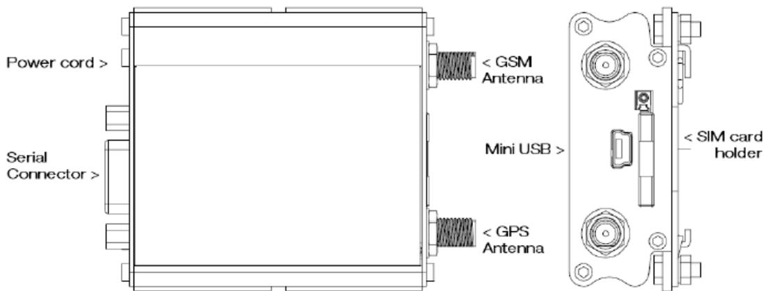
**3. Installing magnetic mount antenna and Power supply.** Connect the mounted cable antenna to the SMA male connector (on your right when facing the connectors) marked "GSM" or "Cellular" on the modem.
