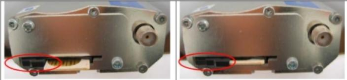
**Warning:** If you're using a GSM modem with an attachable antenna, please exercise caution on attaching the antenna to the antenna connector. If there's a nut attached to the modem casing, please ensure it does not turn when you are connecting the antenna to the modem. Failure to do so may cause damage to the modem.
