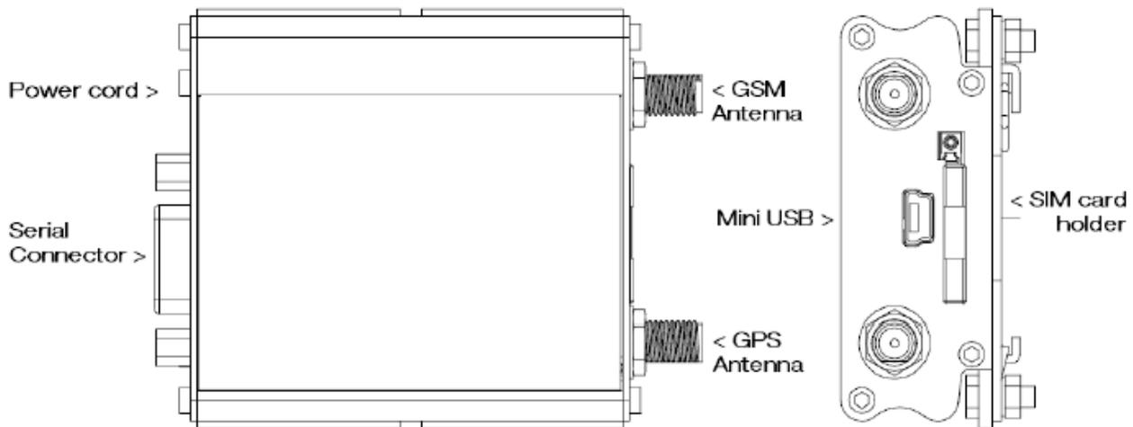
**3. Installing GSM antenna.** Connect the mounted cable antenna to the SMA male connector marked "GSM" on the modem.
