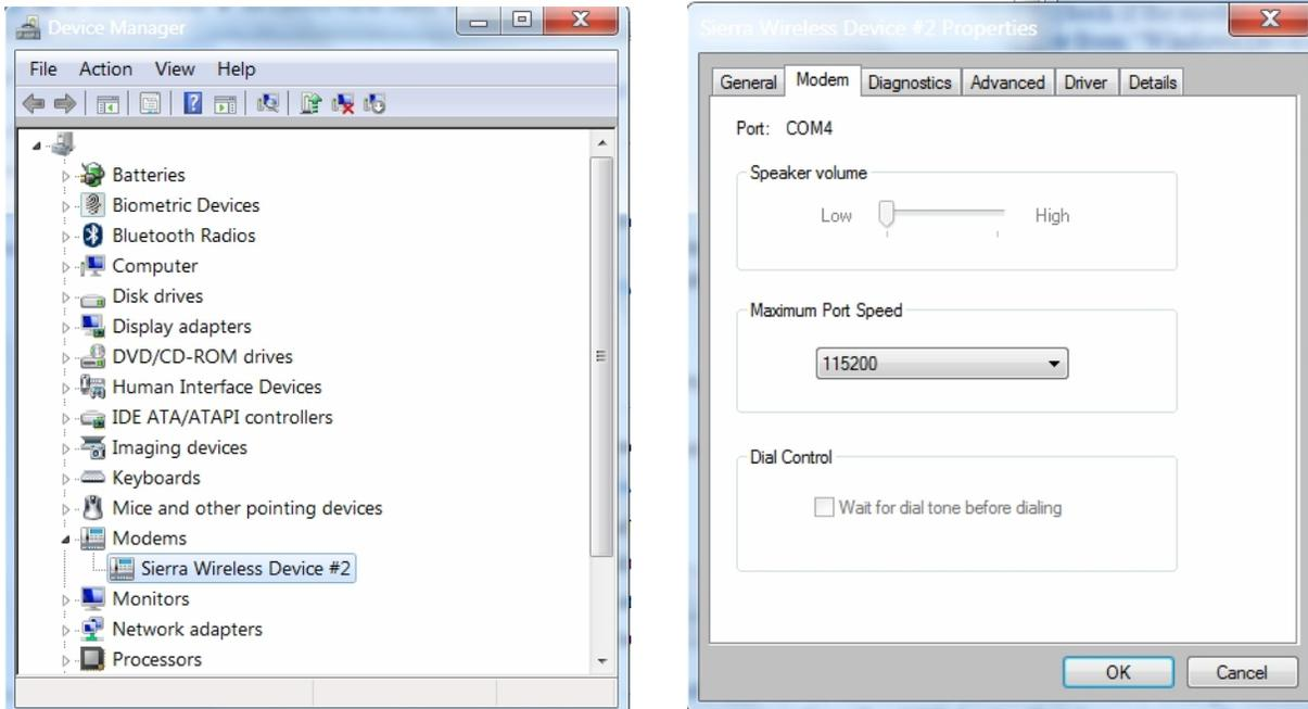
\*Note that the GPRS modem draws considerable USB power so if you are using an USB extension cable or you have connected another USB device that draws too much power (on some PC, power is shared across all the USB ports), the modem may also fail to work or become unstable. You may try removing other USB devices from your PC or using a powered USB hub from a reputable brand such as Belkin.
