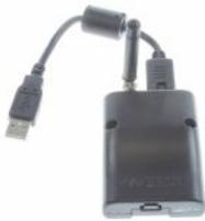
If you are using **Sierra Wireless GL6110 USB modem**, please install the modem driver in your CDROM – path - \Sierra Wireless Modem Driver\XP-2003-2008-Vista-7\USBDriverInstaller.exe.
