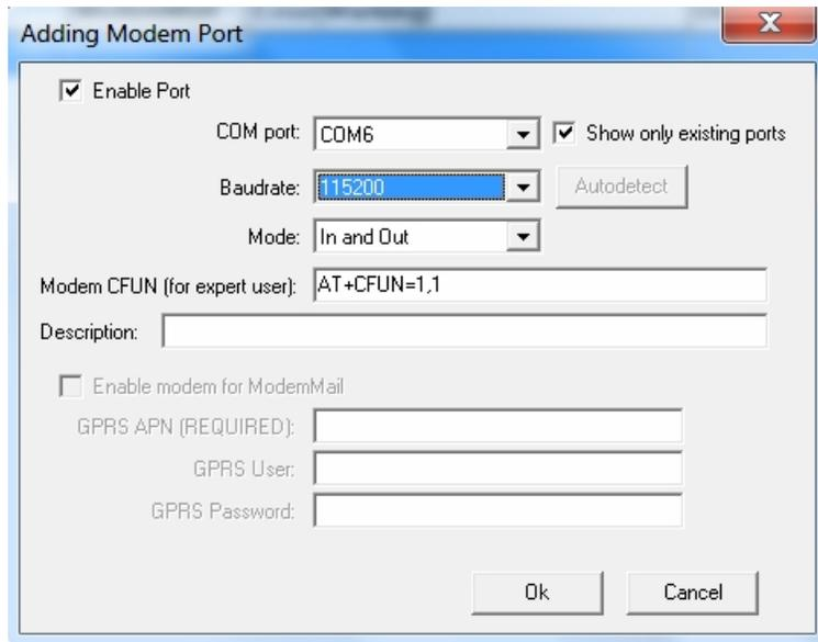
Check ‘*Show only exist ports*’ – this will display only valid COM ports on the system. Select the COM port which your modem is connected to, followed by the baud rate. The most common baud rate is 115200. If unsure, click ‘*Ok*’ button to create the Modem Port, and then select the Modem Port you have just created from
